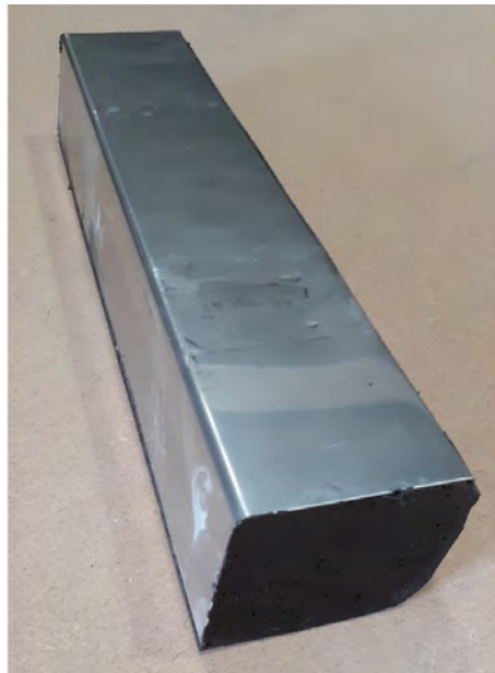
Figure 2: Metal covered Decidamp RTD
