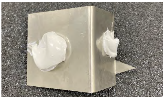
RB Centre Bracket with adhesive applied
